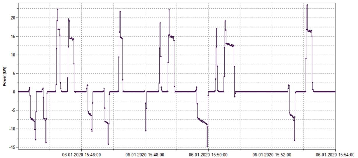
Fig. 8. Power consumption at motor terminal of NRD. NRD, non-regenerative drive.
