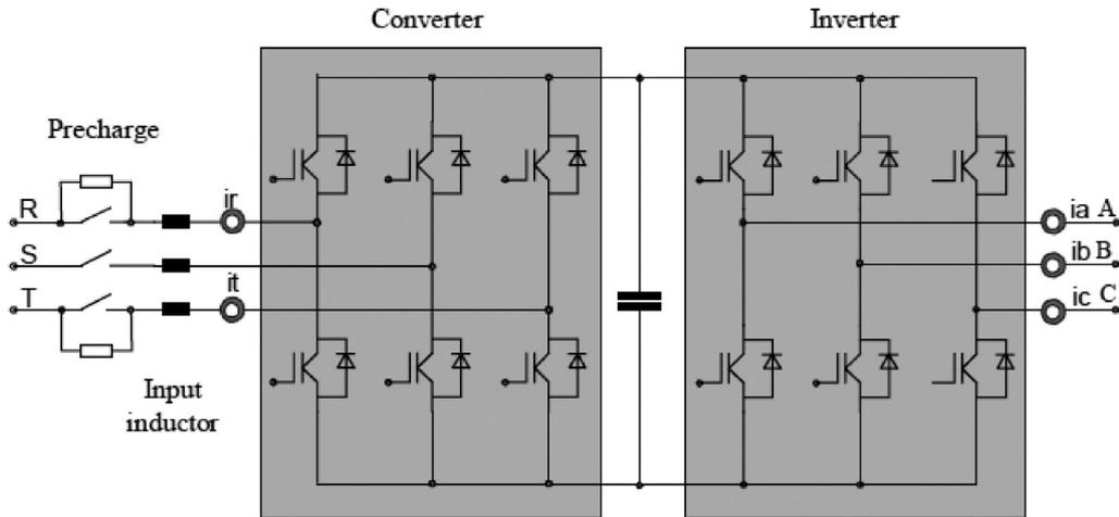
Fig. 3. Schematic Diagram of RDs. RDs, regenerative drives.
