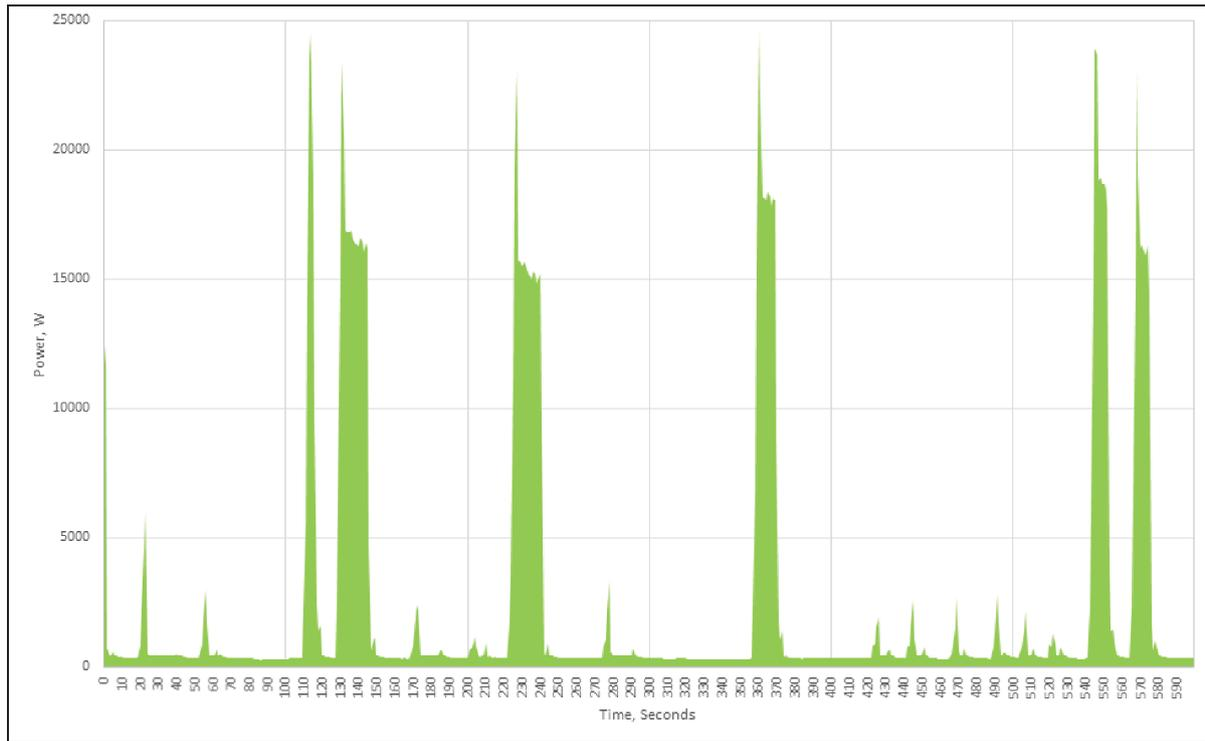
**Fig. 6.** Power consumption measurements in RD during elevator operation. RD, regenerative drive.
