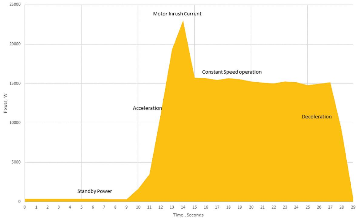
Fig. 7. Energy consumption in NRD in one cycle. NRD, non-regenerative drive.
