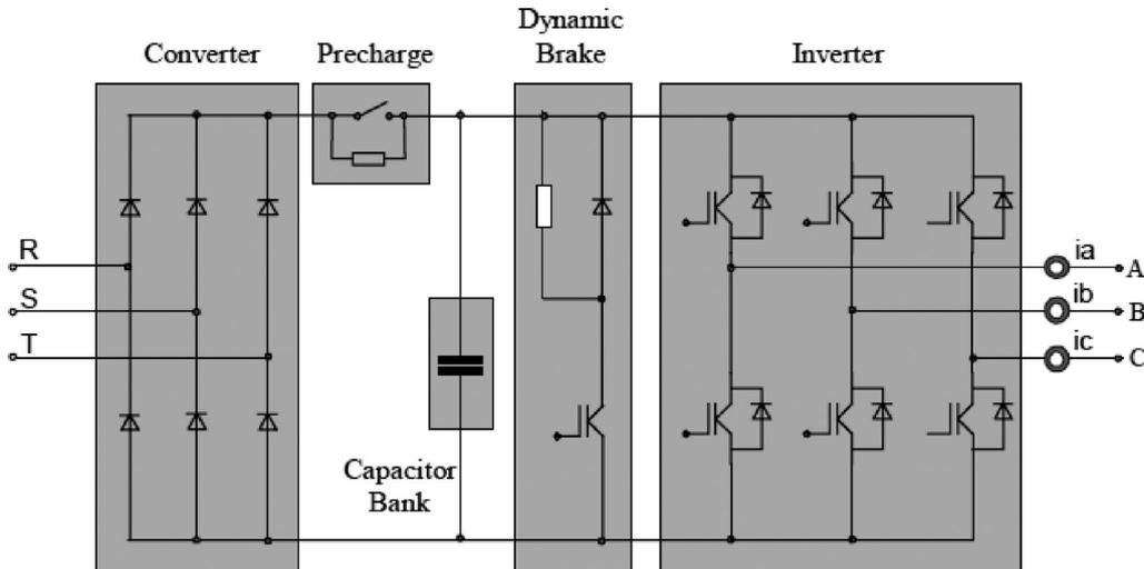
Fig. 4. Schematic Diagram of NRDs. NRDs, non-regenerative drives.
